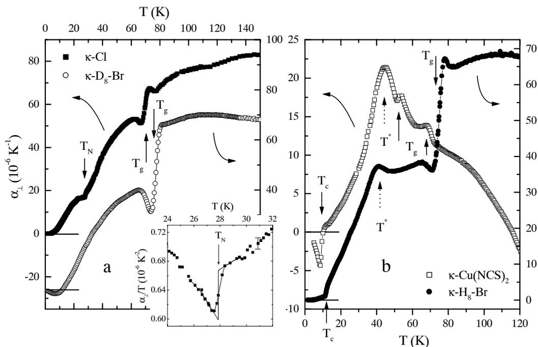
Fig. 1: Cross-plane thermal expansion coefficient for various  $\kappa$ -( $ET$ ) $_2X$  salts;  $H_8$  ( $D_8$ ) indicate protonated (deuterated) ethylene endgroups. Inset shows the phase transition into the AFM ground state for  $\kappa$ -Cl.
