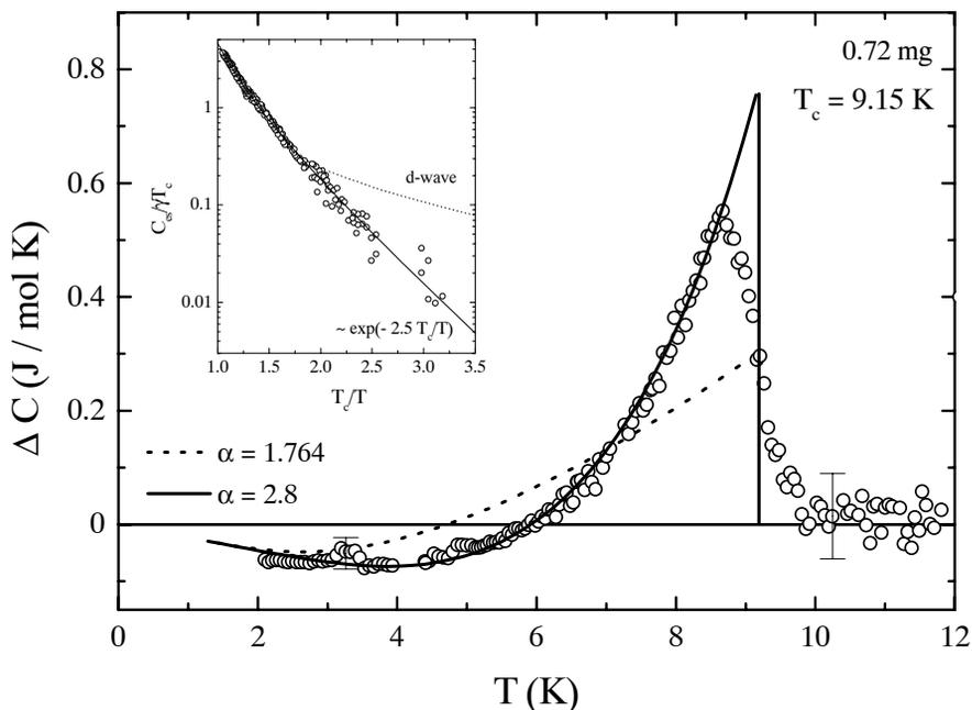
Fig. 4: Specific heat difference  $\Delta C = C(0T) - C(8T) = C(0T) - C_m$ , where  $C_n$  denotes the  $N$ -state specific heat. Dotted and solid thick lines represent BCS curves for weak and strong coupling, respectively. Inset shows the electronic contribution in a BCS-plot.
